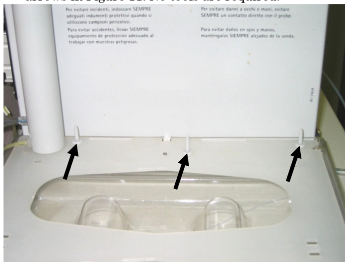
Figure 11. Standards rack locating pins correctly installed.
