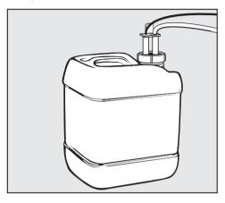
■ Insert the siphon tube into the container and screw on securely (observe the colour code).
