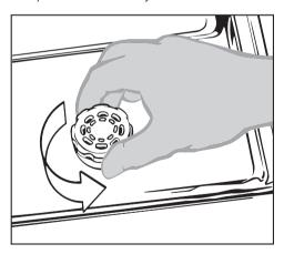
Undo the screw cap.
