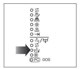
■ Refill the neutralising agent container or replace it with a full container when the Add neutralising agent indicator 🚉 lights up.
