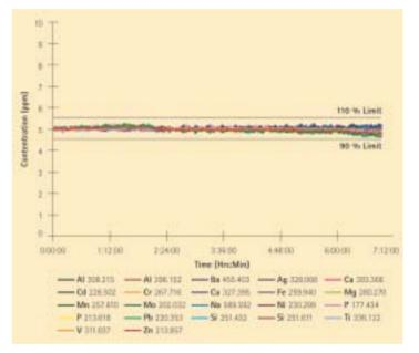
With Varian's unique high solids torch, the axial Vista-PRO shows excellent stability for the direct aspiration of 25% sodium chloride over 24 hours. (Top) The stability of elements in kerosene directly aspirated for 8 hours with no internal standardization is shown. (Bottom)
