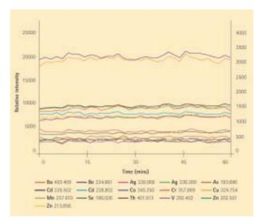
The direct aspiration of methanol for an extended period is a test of RF and sample introduction stability. This continuous measurement of a range of elements for over an hour demonstrates the excellent robustness and stability of the Vista-PRO.
