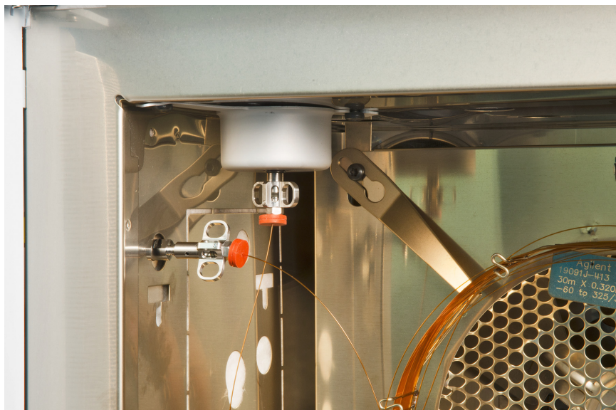
Figure 23. Installing a capillary column in the GC/MSD interface
