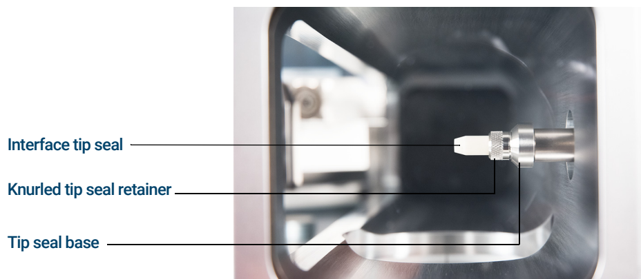
Figure 17. GC/MSD interface tip seal
