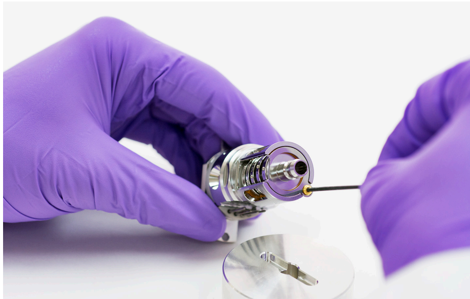
Figure 60 Secure the lens screw and lock ring insulator
