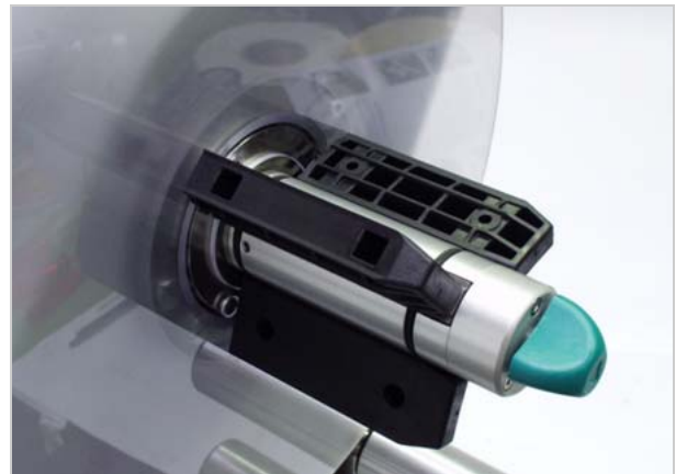
[48] Core adapter positions for a core diameter of 101.6 mm.
