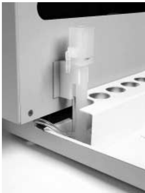
Figure 3-9. View of rinse station.
