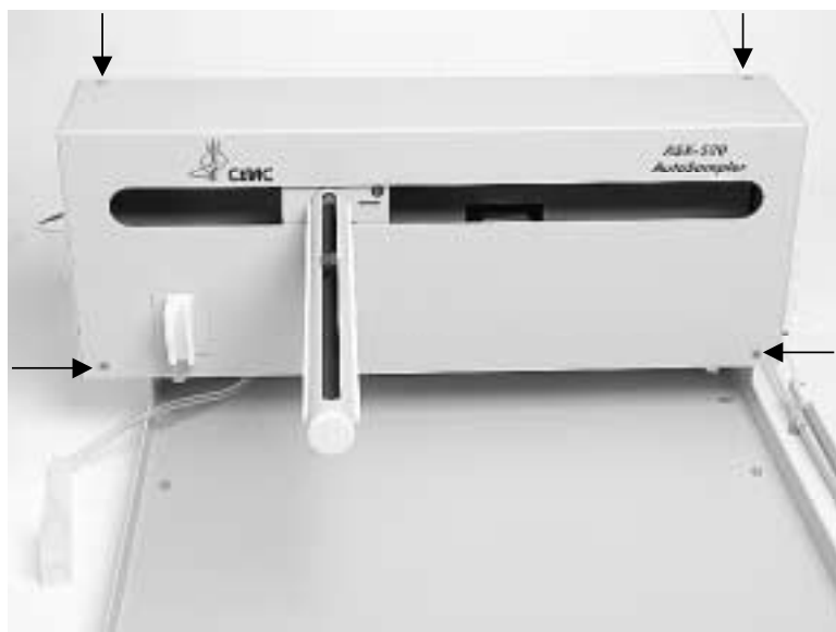
Figure 3-12. Front view of ASX-520 Autosampler showing front cover screws.
