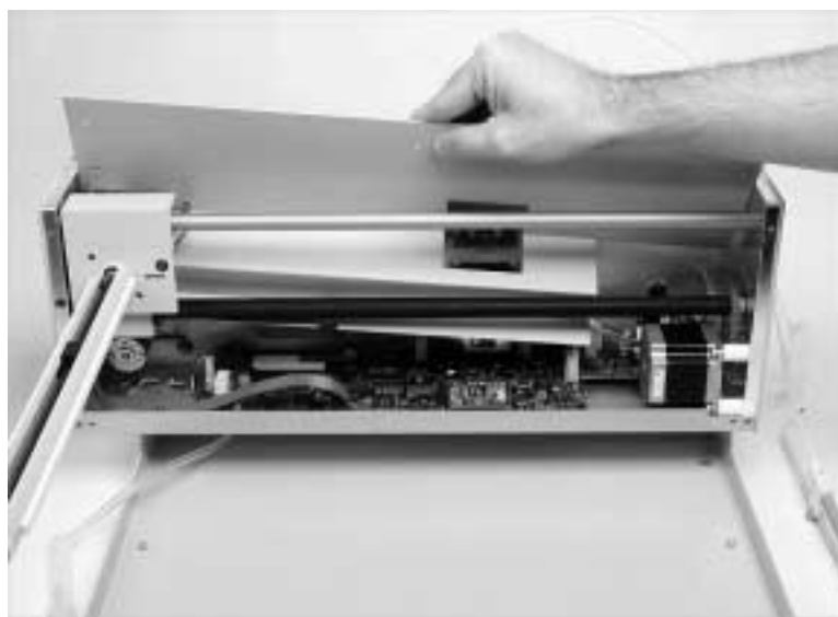
Figure 3-15. Removal of inner shield.
