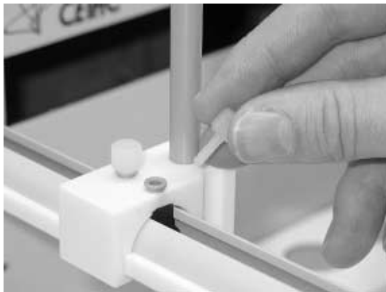
Figure 3-7. View of Y- axis home block with Kynar thumbscrews.
