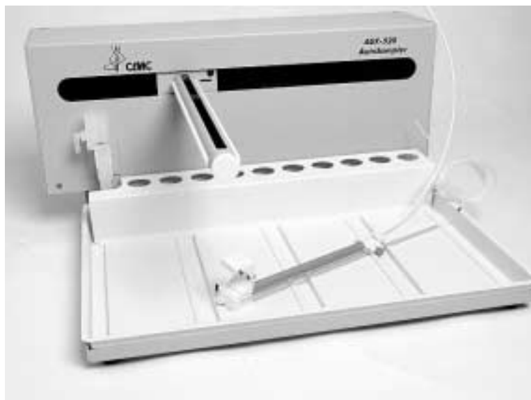
Figure 3-8. Z-drive removed from arm assembly.
