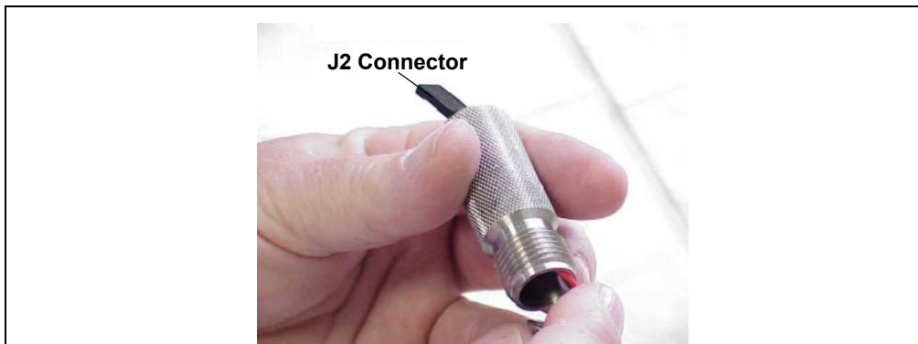
Figure B-10. Installing the Electrode Cylinder
