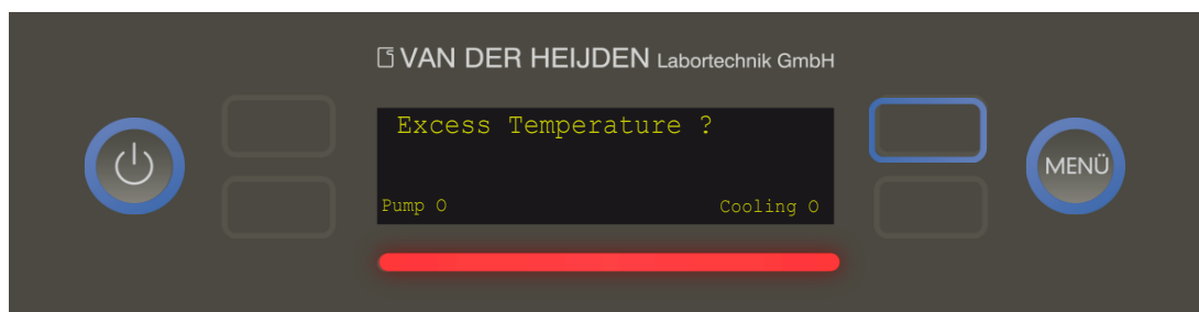
-Fig. 9: Disruption – 'Excess temperature rise alarm'
