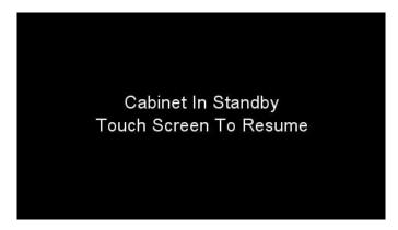
Touching the screen will wake the cabinet , open the sash, start the fans and resume operation.
