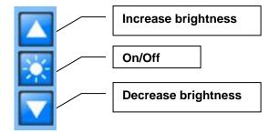
By pressing the *"Up"* or *"Down"* arrows you can adjust the brightness. Pressing the *"Lighting"* icon will turn the light off. Pressing the icon again will turn the light on.
