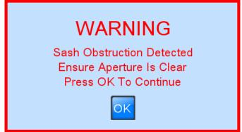
Remove the obstruction and press "OK". This will reset the system and the sash will close.
