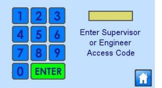
Press "0127" then "*Enter*" to start the cabinet. The screen will move to calibrate the sash closed position. It will then automatically open the sash to its normal working position, the fans will start and the lighting will illuminate.
