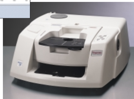
Nicolet 380 with a Smart SAGA™ Grazing Angle Accessory
