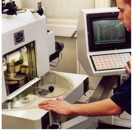
Figure 18.4 LEFT: Diamond turning machine; RIGHT: Lens polishing
