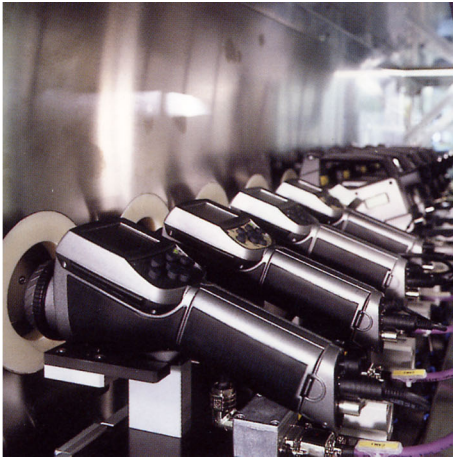
Figure 18.5 LEFT: Testing of infrared cameras in the climatic chamber; RIGHT: Robot used for camera testing and calibration
