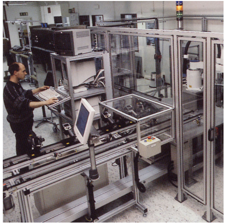
Figure 18.5 LEFT: Testing of infrared cameras in the climatic chamber; RIGHT: Robot used for camera testing and calibration
