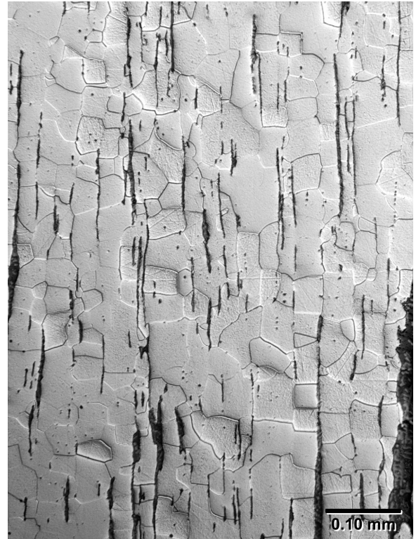
Figure 7. Wrought iron from a 19 th century train. (Labophot 2A, 10X objective, differential interference contrast.)
