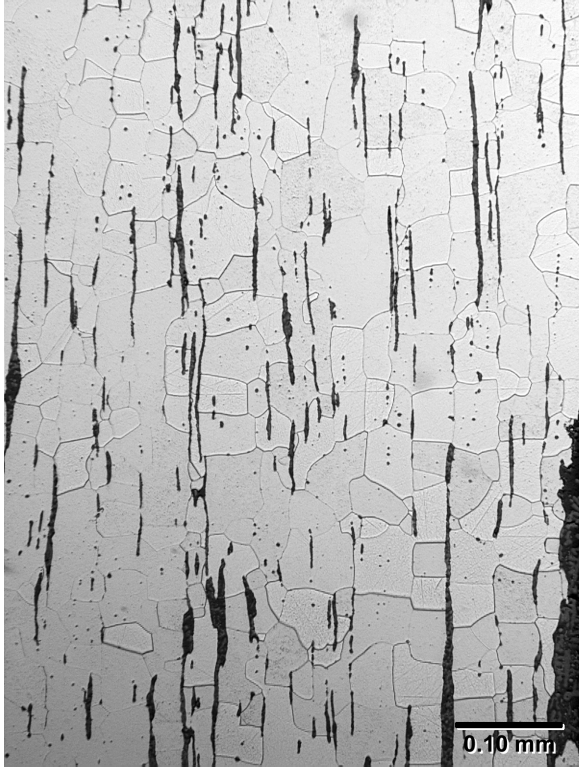
Figure 4. Wrought iron from a 19 th century train. (Labophot 2A, 10X objective, bright field illumination.)
