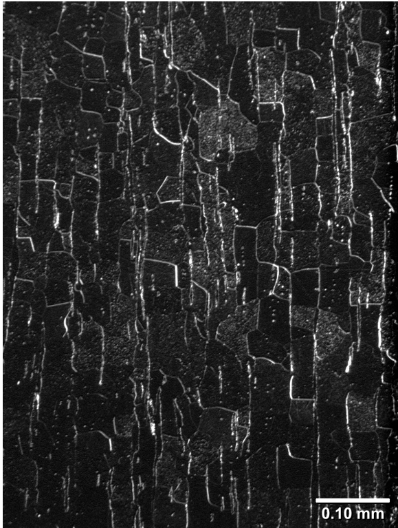
Figure 6. Wrought iron from a 19 th century train. (Labophot 2A, 10X objective, dark field illumination.)
