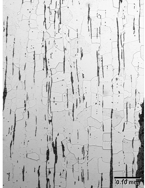
Figure 5. Wrought iron from a 19 th century train. (Labophot 2A, 10X objective, polarized light.)
