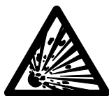
Risk of explosion
