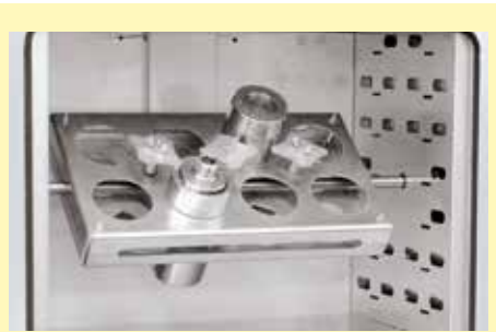
Electrical rotating device (in this case with tailored platform for PARR autoclave containers)
