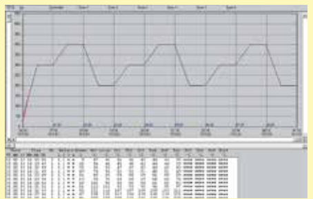
Software for documentation of the temperature curve and combustion loss using a PC
