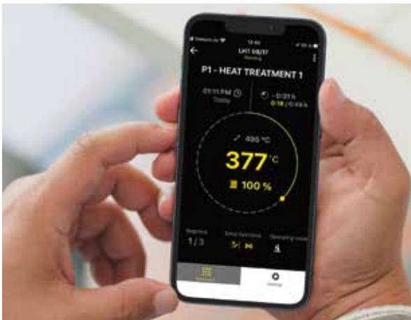
Display of program progress for each furnace
