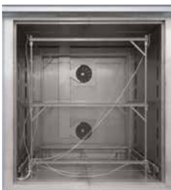
Pluggable frame for measurement for forced convection chamber furnace N 7920/45 HAS
