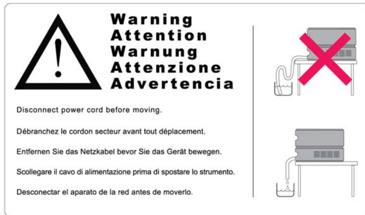
Figure 23 Warning label (illustration for correct waste tubing)
