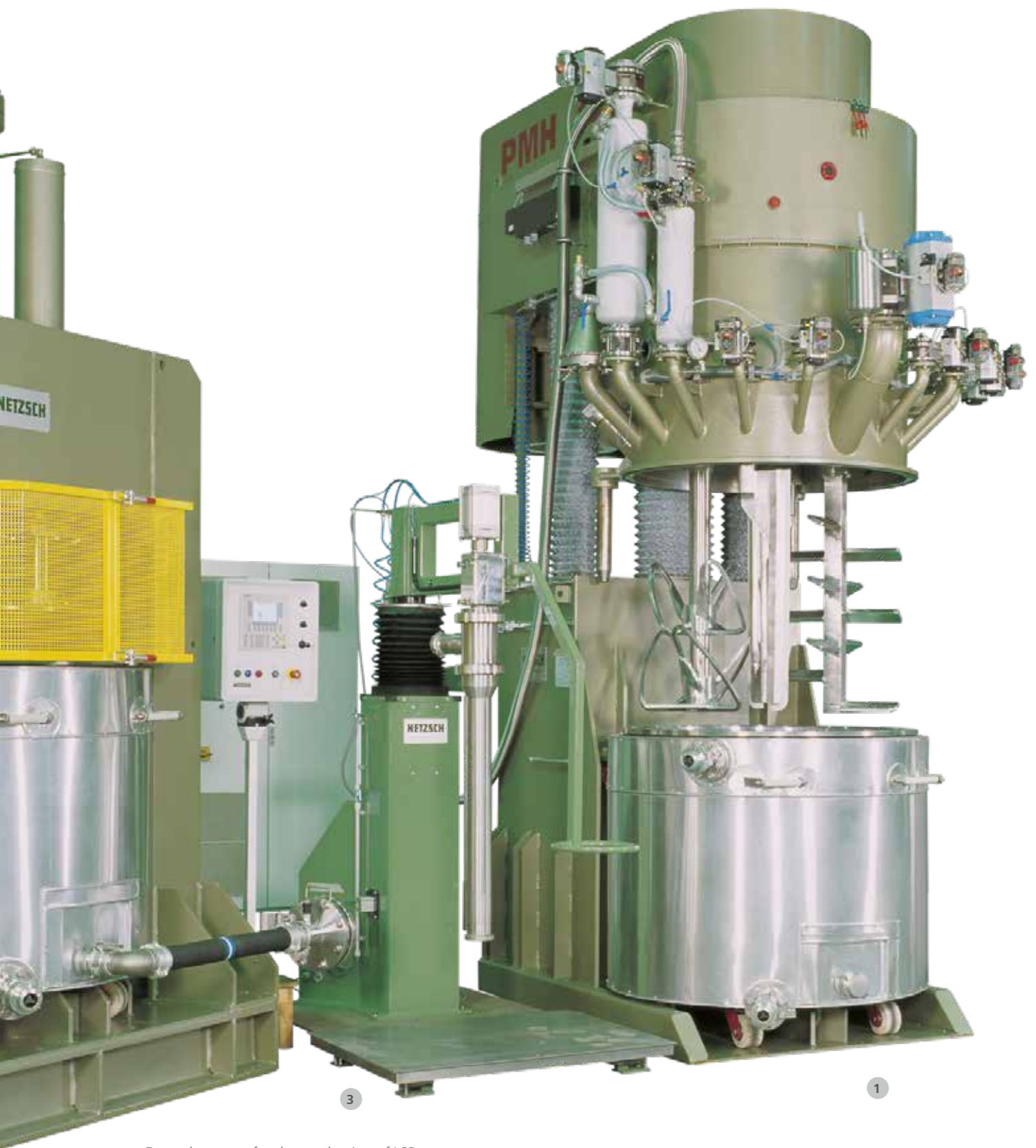
Example system for the production of LSR
