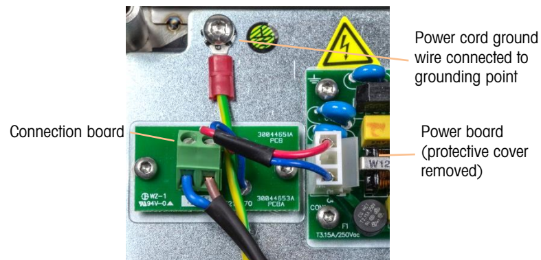
Figure 2-18: IND236 AC Power Connection Board and Grounding
