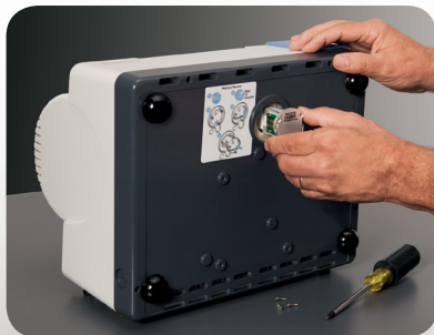
Infrared source replacement
