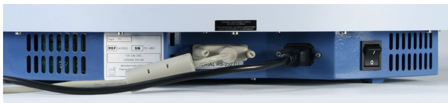
Figure 3–14. Mains supply cable and serial cable connected
