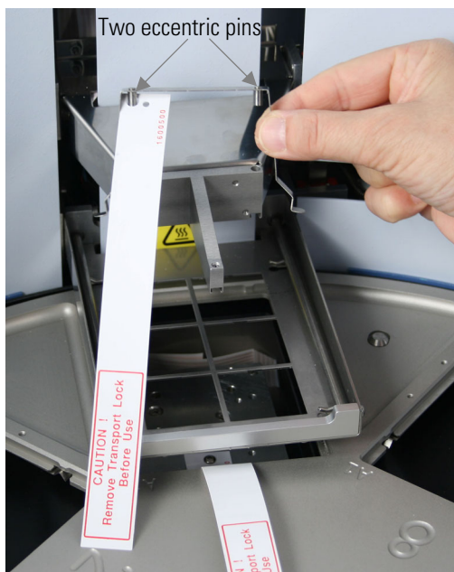
Figure 3–11. Tip comb holder transport lock removed
