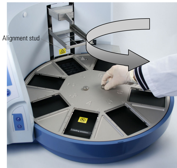
Figure 5–49. Unfastening the two finger screws
