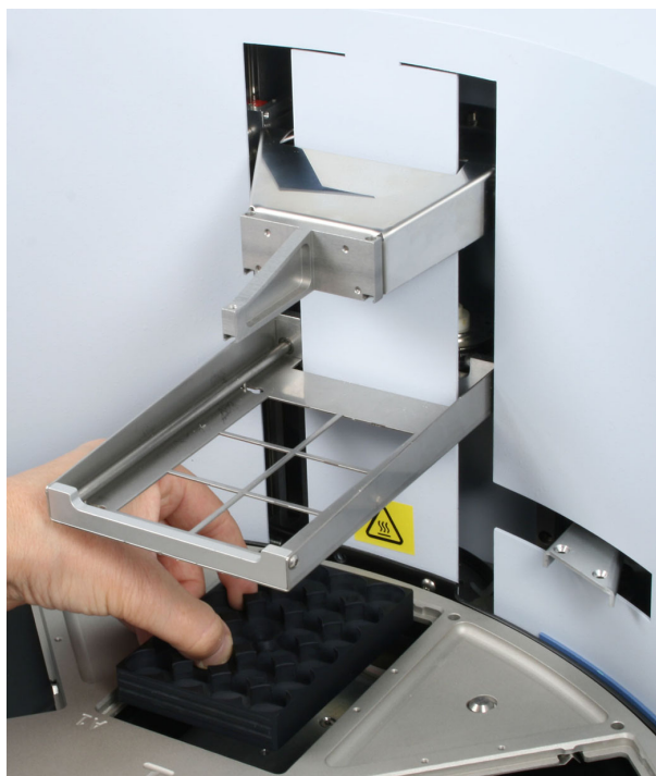
Figure 4–46. Inserting the heating block
