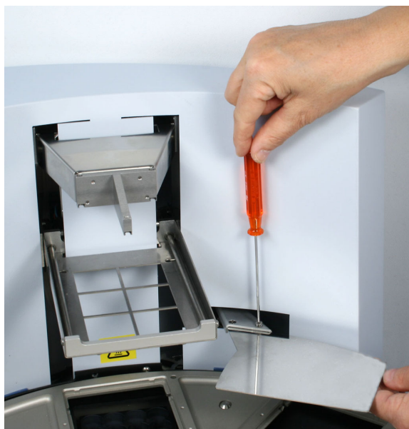
Figure 3–20. Fastening / loosening the shield plate
