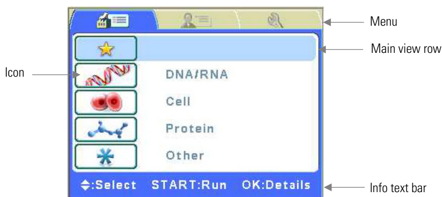
Figure 4–32. Main view on the display of the KingFisher Flex
