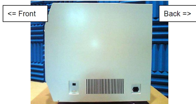
Figure 3. Right-side view of the instrument showing the position of Power Inlet Connector and the Fuse Unit.
