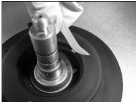
Removing plastic debris with tape.
