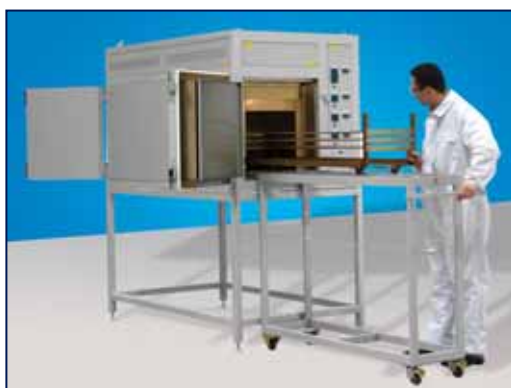
A PASS THROUGH CLEAN ROOM OVEN WITH CUSTOM LOADING SYSTEM FOR MEDICAL DEVICE MANUFACTURE
