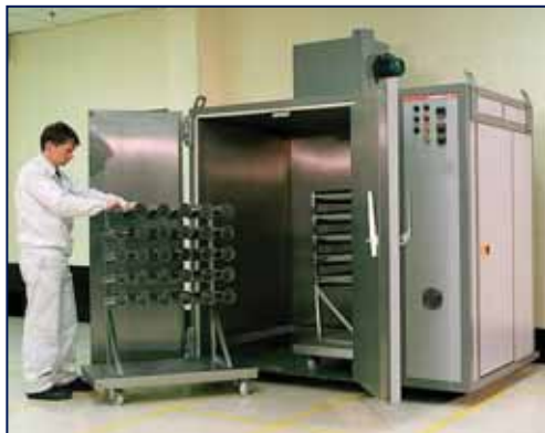
A BESPOKE LGP OVEN FOR HEAT TREATMENT OF LASERJET PRINTER IMAGING DRUMS
