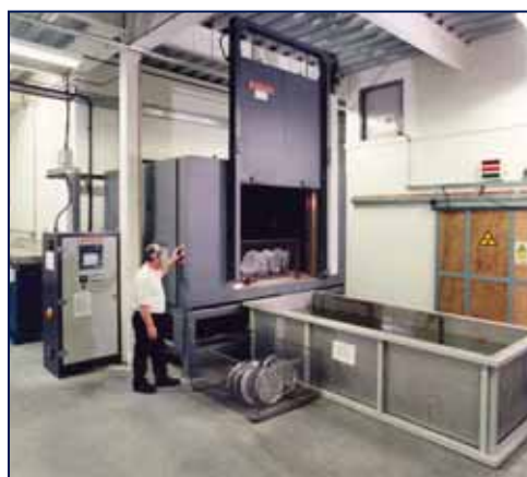
CUSTOM BUILT 300°C LGP OVEN WITH DROP QUENCH
