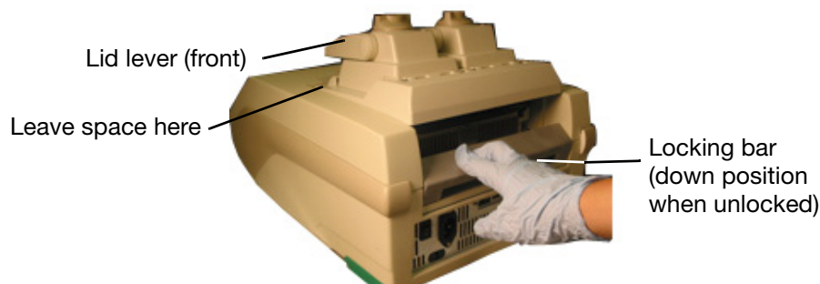
Figure 6. Inserting the reaction module into the bay.
