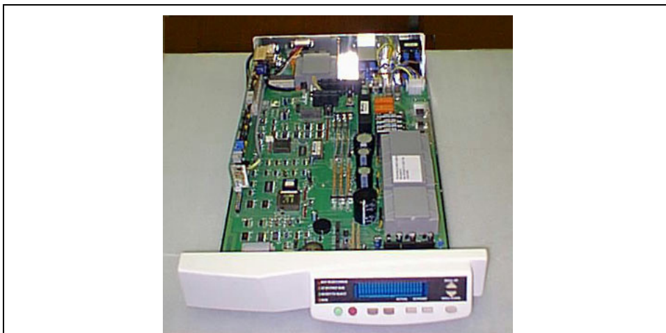
Figure 1-5. Example of Electronic Compartment
