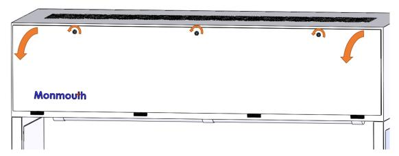
• Working inside the enclosure, in turn, slacken the 2 off screws (17mm A/F) clamping each fan box module to the filter. Work each side in turn to raise the fan box evenly until a sufficient gap is present to enable the removal of the HEPA filter which should freely slide out of place.
