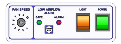
The booth is started by first operating the Green rocker switch on the control panel. The Red airflow monitor warning light will flash until the correct airflow is achieved.
