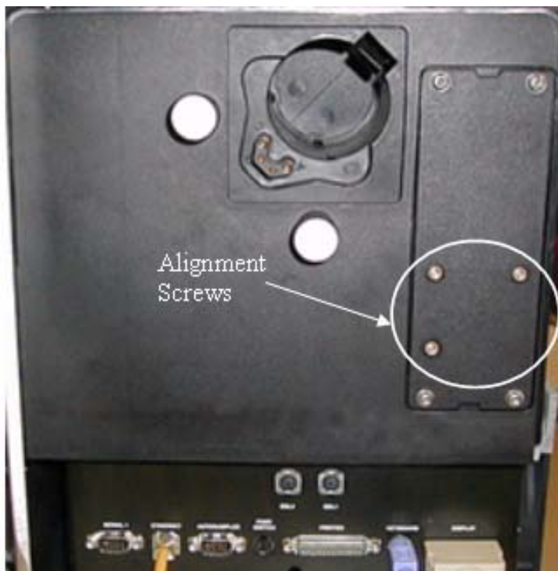
Figure 9-19 Location of the alignment screws of the deuterium lamp.
