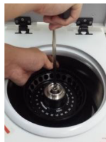
Picture 9 Tool for rotor without nut
